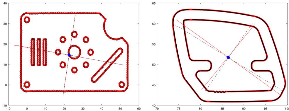
Fig. 4. Point-cloud comparison for the details: Red(solid): (Fuzzed) CAD sample and its KL frame. Black(circled): Scanned data and its KL frame. Blue dots: Barycenters
