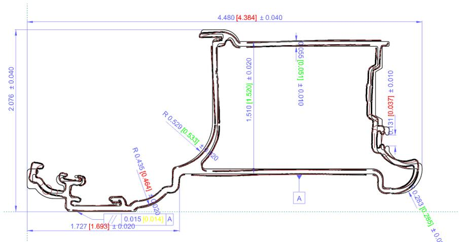
Fig. 1. CAD vs. CAM comparison of an industrial detail. Green numbers pass the quality inspection, while red ones do not
